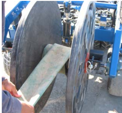
Typical method of storage. Retrieving on the layflat spool. Layflat Spool sizes: 4”, 6”, & 8”
