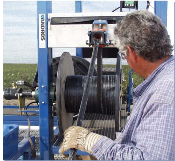
RH03-100C Linear Tape Counter Traverse Arm Assembly
